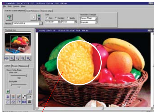
Loupe tool Zooms an area of interest for closer inspection. Can be moved freely around the entire image, with selectable magnification.
